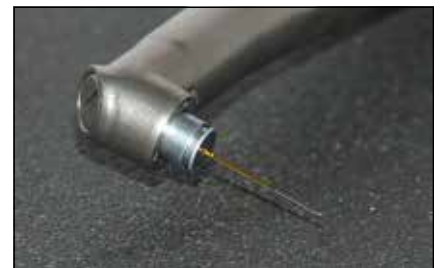
Fig. 2. PIPS tip in laser handpiece showing the stripped and radial firing tip.
